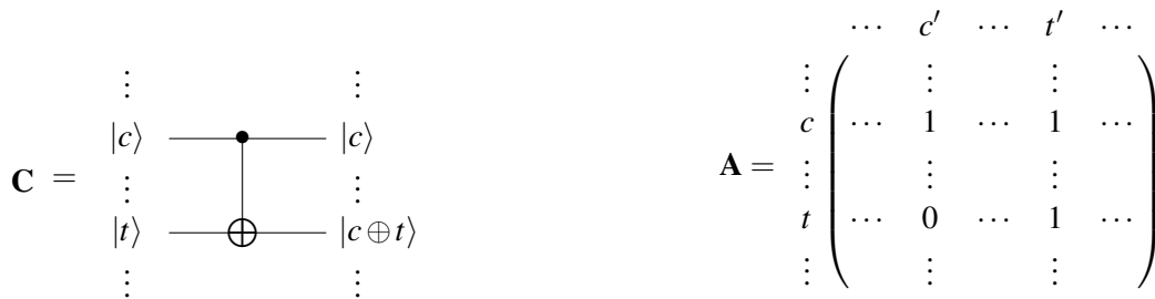
(a) \mathbf{C} is an n -qubit CNOT circuit with one CNOT gate.
